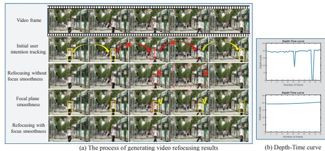
**Fig. 4.** The comparison between video refocusing without and with focal smoothness, (a) illustrates the initial tracking results of user intention and the improved effects by utilizing focal plane smoothness, red rectangle means missing match while yellow is the correct tracking results, and (b) is the depth-time curve before and after focal plane smoothness.
