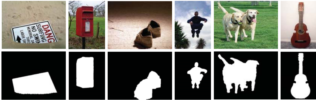
Fig. 1 Examples of images in MSRA10K dataset. (top row) Source images. (bottom row) Corresponding manually labeled ground truths.
