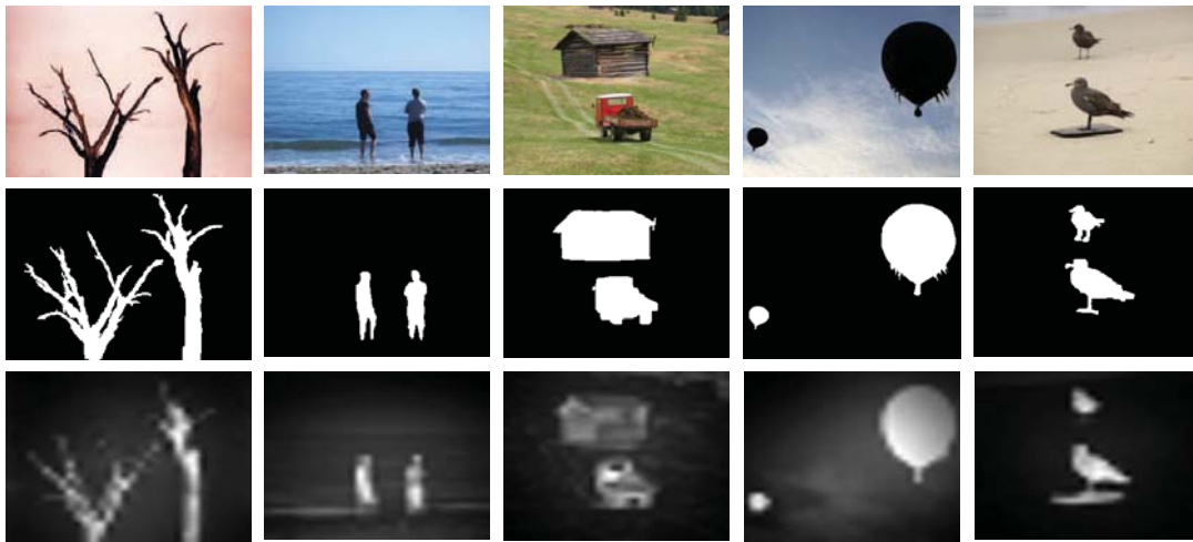
Fig. 18 Examples of saliency maps generated by LSP using different patch decomposition on SED2 dataset. (top row) Source images. (middle row) Ground truths. (bottom row) Saliency maps generated by LSP 32 \times 32 .
